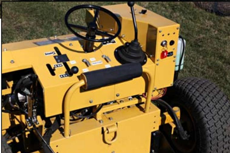
Meet Magnum's latest Installer, the turf and operator friendly, four-wheel drive machine that combines efficiency and dependability into a conveniently compact package weighing less than 2000 pounds. The concept of this Installer grew out of the need for a lighter weight, quick moving vehicle for the installation of big rolls of sod, one that could handle the terrain but not damage the turf.
