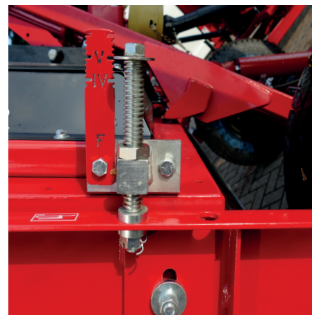
The height of cut is easily adjusted from 13 to 100 mm.
