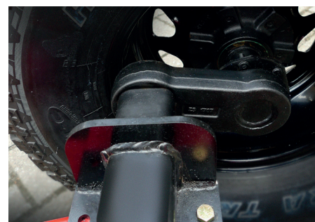
Shock absorbing torsion suspension.
