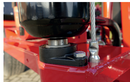
Maintenance free sealed bearings in both the blade spindles and roller ends.
