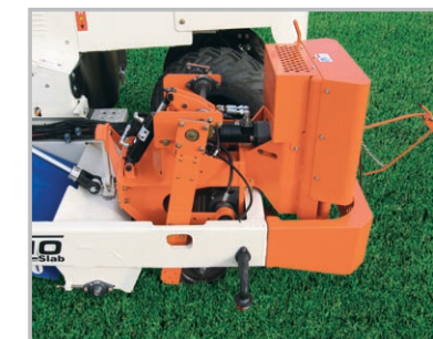
Floating cutting head with adjustable-down pressure
